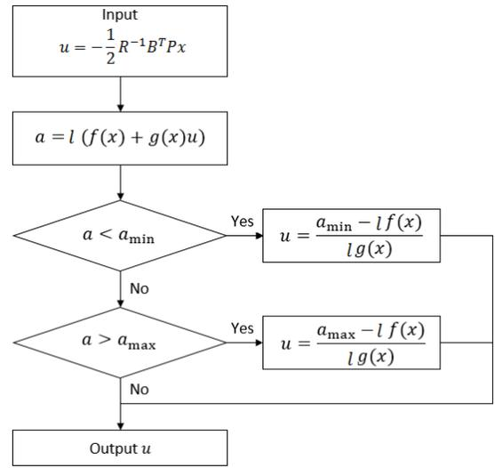
Figure 3 Input modification algorithm to satisfy acceleration constraint for LQ controller.
