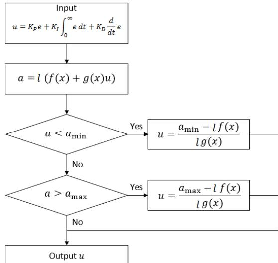
Figure 7 Input modification algorithm to satisfy acceleration constraints for PID controller.
