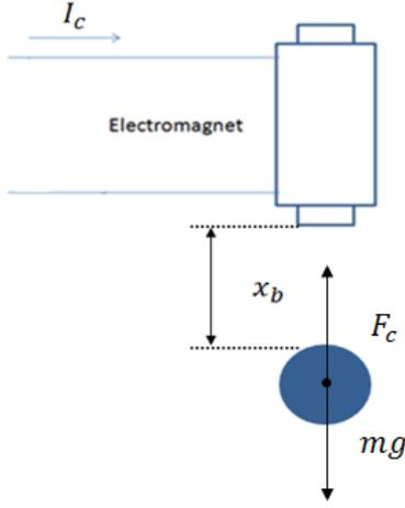
Figure 1 Schematic Diagram of Magnetic Levitation System
