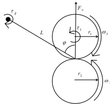
Figure 1 Simplified Diagram of the ABS Experimental Device
