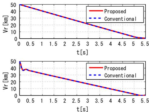
Figure 4 Car Velocity On Dry Road
