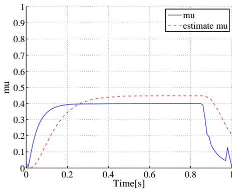
Figure 8 Comparison of the friction coefficient
