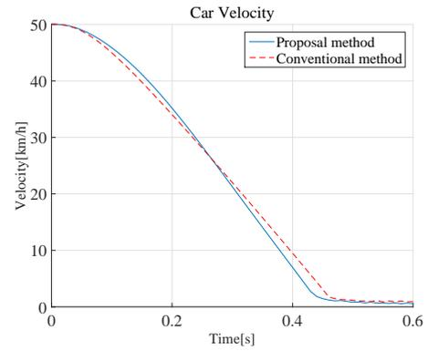
Figure 9 Comparison of the car velocity at the dry road
