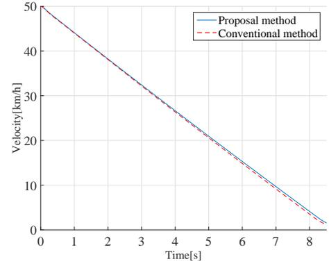
Figure 3 Comparison of the car velocity at the frozen road
