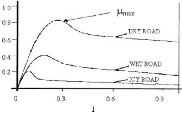
Figure 2 Comparison of slip rate
