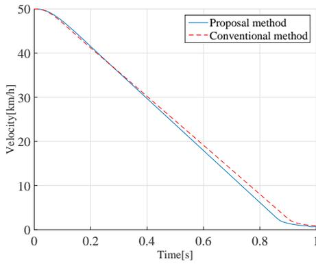
Figure 6 Comparison of the car velocity at the wet road
