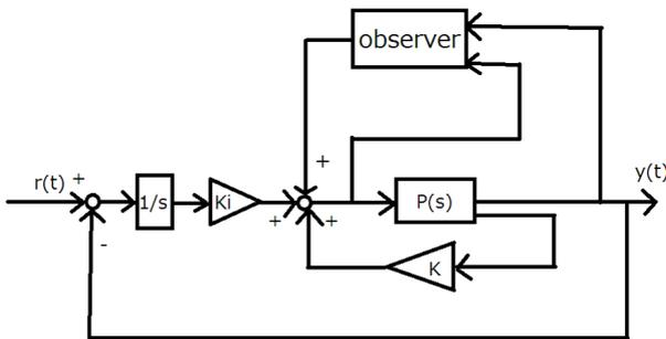
Figure 1 Robust  $H_2$  control system with full order observer
