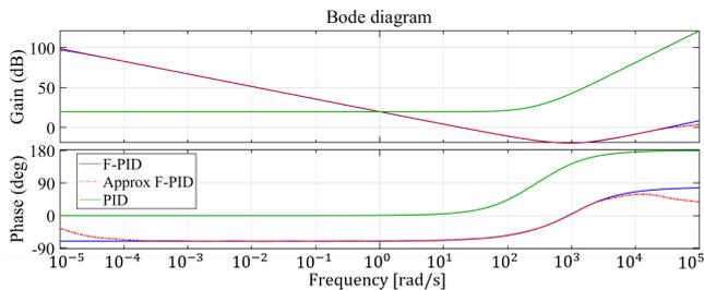
図 7 Bode diagram of controllers
