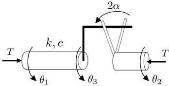
図1 Backlash system: a shaft connected to a backlash
