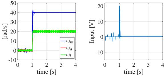
図 5 Time response of fractional PID control
