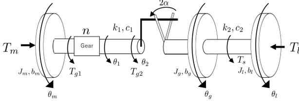
図3 The three-inertia model
