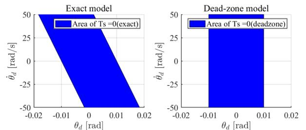
図2 Phase plane ( $\theta_d - \dot{\theta}_d$ ):  $\alpha = 0.01$  [rad],  $k/c = 6000$  [s<sup>-1</sup>]
