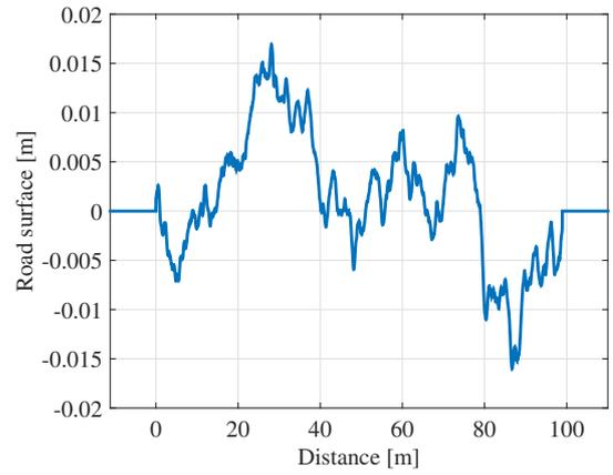
Figure 4 Road surface for ISO8608 Class:A
