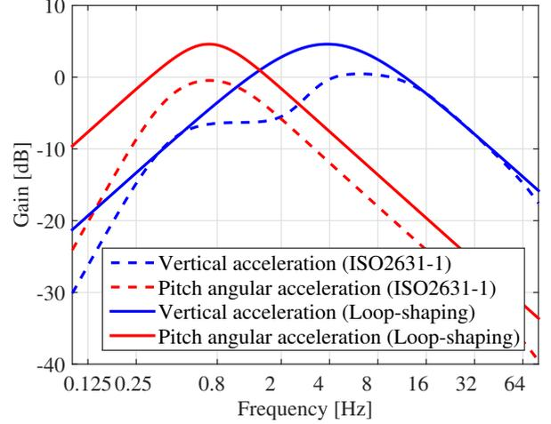
Figure 2 Frequency weight for ISO2631-1 and loop-shaping
