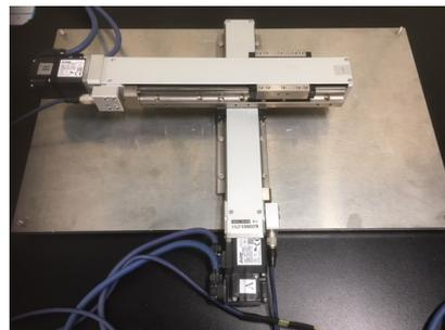
Figure 1 Ball Screw System
