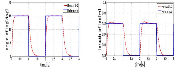
Fig. 7 Angle of support leg Fig. 8 Length of support leg and swing leg
