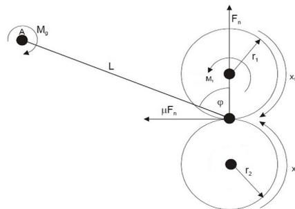
Figure 2 Physical Model of ABS
