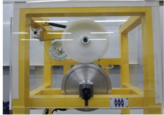
Figure 1 ABS Experimental Unit
